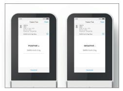
**8.** Results are displayed within 5 minutes of applying the sample. The left-hand image here shows a positive result for SARS-CoV-2 Ag and the right-hand image shows a negative result for SARS-CoV-2 Ag. Tap Finish to complete testing or tap Comment to leave a comment or to reject the Test, then follow prompts to return to the Home Screen. All test results must be read using the LumiraDx Instrument.
