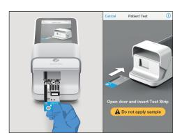
3. When prompted, open the Instrument door and gently insert the Test Strip as far as it will go. The thick black alignment rib on the Test Strip should be on the left and line up with the black line on the Instrument. Do not apply the sample until prompted. Install the Lot Calibration file if using a new Test Strip Lot for the first time. See section 2.8 of the Platform User Manual.
