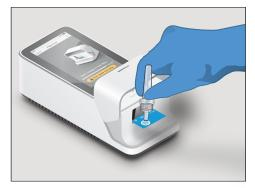
Apply one whole drop of the sample onto the Test Strip Sample Application Area when prompted by the Instrument.
