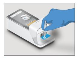
7. Squeeze the Extraction Vial to apply one whole drop of the sample onto the Test Strip Sample Application Area when prompted by the Instrument.
