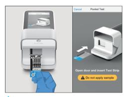
4. When prompted, open the Instrument door and gently insert the **Test Strip** as far as it will go. The thick black alignment rib on the **Test Strip** should be on the left and line up with the black line on the Instrument. **Do not apply the sample until prompted.** Install the Lot Calibration file if using a new **Test Strip Lot** for the first time. See section 2.8 of the **Platform User Manual**.
