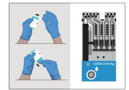
**3.** Remove the **Test Strip** from its pouch and hold by gripping only the blue portion. **Do not bend the Test Strip or touch any part other than the blue portion.**
