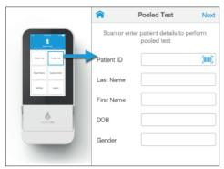
**1.** Select *Pooled Test* from the **Instrument** *Home Screen* and enter the first individual sample information in the Patient ID details using the **Keyboard** then press *Next*.
