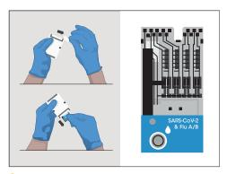
2. Remove the Test Strip from its pouch and hold by gripping only the blue portion. Do not touch the Test Strip Sample Application Area. Do not bend the Test Strip or touch any part other than the blue portion.
