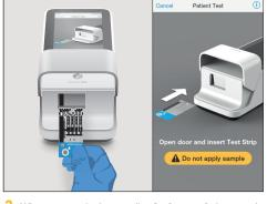
3. When prompted, open the Instrument door and gently insert the Test Strip as far as it will go. The thick black alignment rib on the Test Strip should be on the left and line up with the black line on the Instrument. Do not apply the sample until prompted. Install the Lot Calibration file if using a new Test Strip Lot for the first time. See the Platform User Manual for further details.
