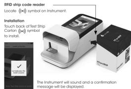
When indicated by the touchscreen open the foil pouch just before use and insert the LumiraDx Test Strip into the LumiraDx Instrument. The Instrument will indicate when it is ready for the sample to be applied.
