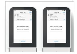
**9.** Results are displayed within 5 minutes of applying the sample. The left-hand image here shows an Ultra pooled positive result for SARS-CoV-2 Ag and the right-hand image shows a pooled negative result for SARS-CoV-2 Ag.
