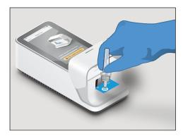
Squeeze the Extraction Vial to apply one whole drop of the sample onto the Test Strip Sample Application Area when prompted by the Instrument.
