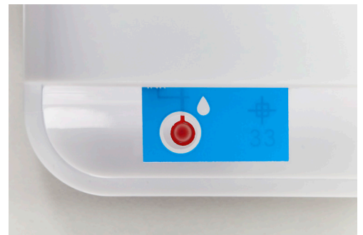
Insufficient sample applied.
