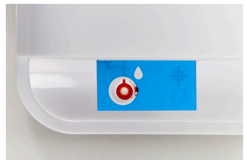
Air bubbles in Sample Application Area.
